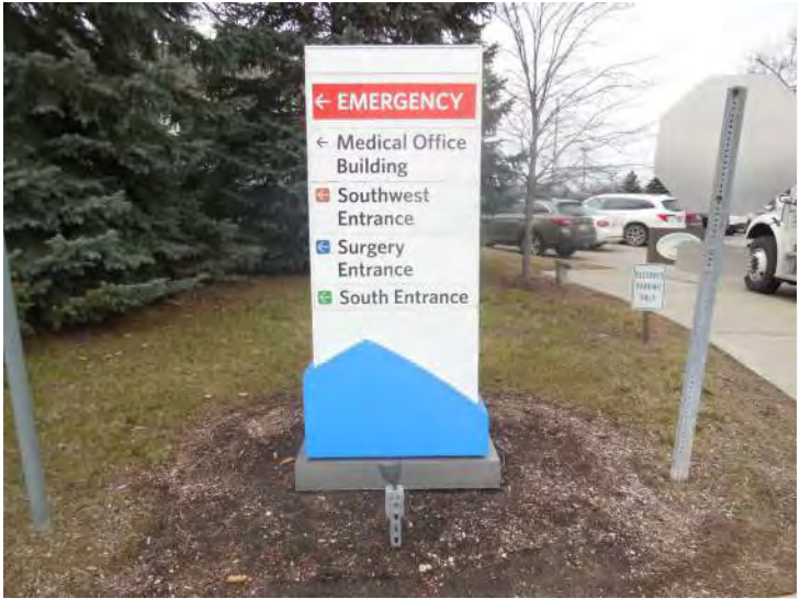
Existing 7'-3" x 2'-6" signage to be removed & replaced; Re-use existing electrical; Installed far enough away to avoid existing footer
