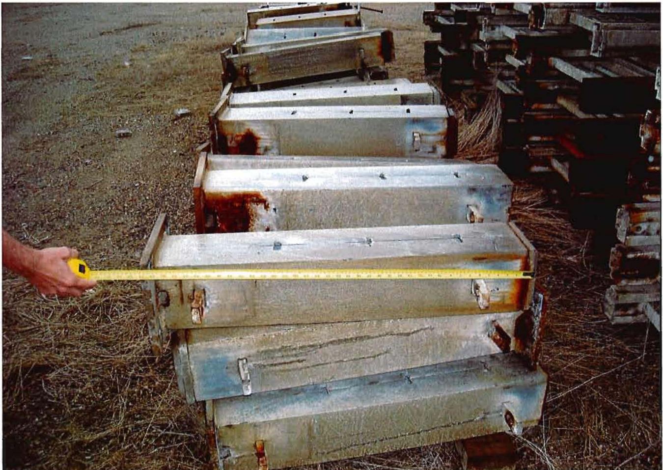
PHOTO 4 MDOT SALVAGED STEEL POSTS FOR VINTAGE RAILING
