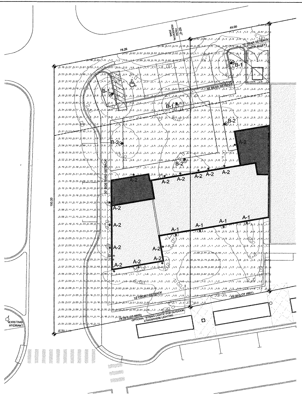
1 SITE LIGHTING PHOTOMETRIC PLAN SCALE: 1" = 10'
