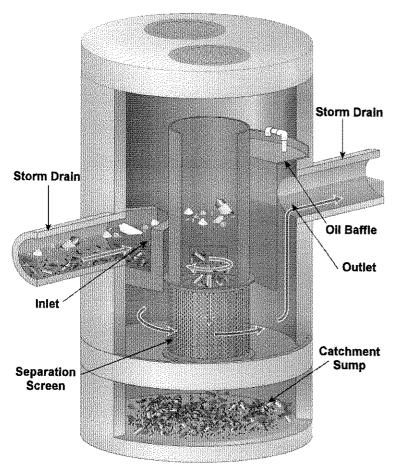
The visual inspection should ascertain that the unit is functioning properly and that there are no blockages or damage to the inlet, separation chamber or separation screen. The quantities of captured pollutants within the separation chamber and solids storage sump should be assessed.
