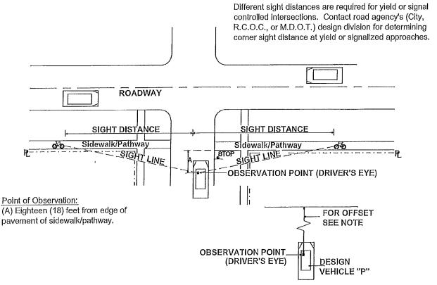
The point of vision shall be from the height of eye, 3.5 feet above the proposed intersecting elevation to a height of object 3.5 feet above the existing or proposed road centerline and shall be continuously visible within the specified limits.
