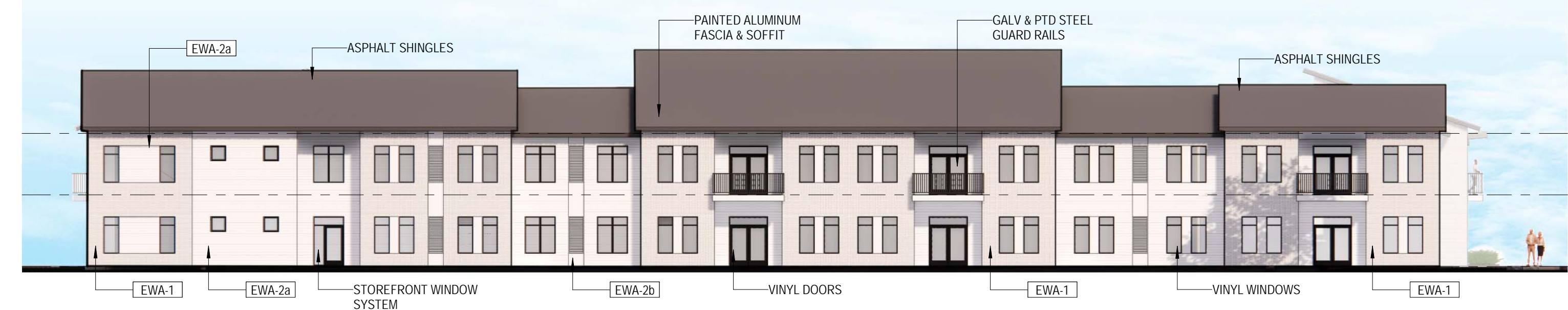
2 | ENLARGED WEST ELEVATION (EAST ELEVATION OPPOSITE HAND)
