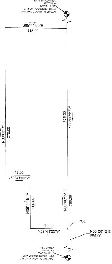
PART OF SE 1/4, OF T3N, R11E, SEC 6, BEGINNING AT PT DISTANT N 00°06'15" E 655.00 FT FROM SE CORNER, THENCE N 89°41'00" W 70.00 FT, THENCE N 00°06'15" E 100.00 FT, THENCE N 89°41'00" W 45.00 FT, THENCE N 00°06'15" W 275.00 FT, THENCE S 89°41'00" E 115.00 FT, THENCE S 00°06'15" E 375.00 FT, TO THE POINT OF BEGINNING.
