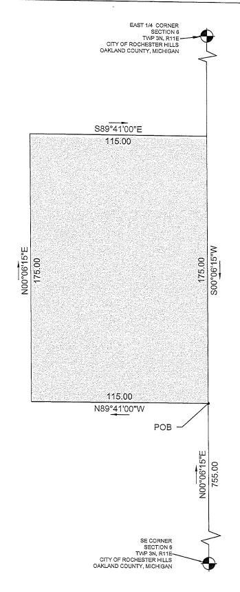
PART OF SE 1/4, OF T3N, R11E, SEC 6, BEGINNING AT PT DISTANT N 00°06'15 E 755.00 FT FROM SE CORNER, THENCE N 89°41'00" W 115.00 FT, THENCE N 00°06'15" E 175.00 FT, THENCE S 89°41'00" E 115.00 FT, THENCE S 00°06'15" E 175.00 FT, TO THE POINT OF BEGINNING.
