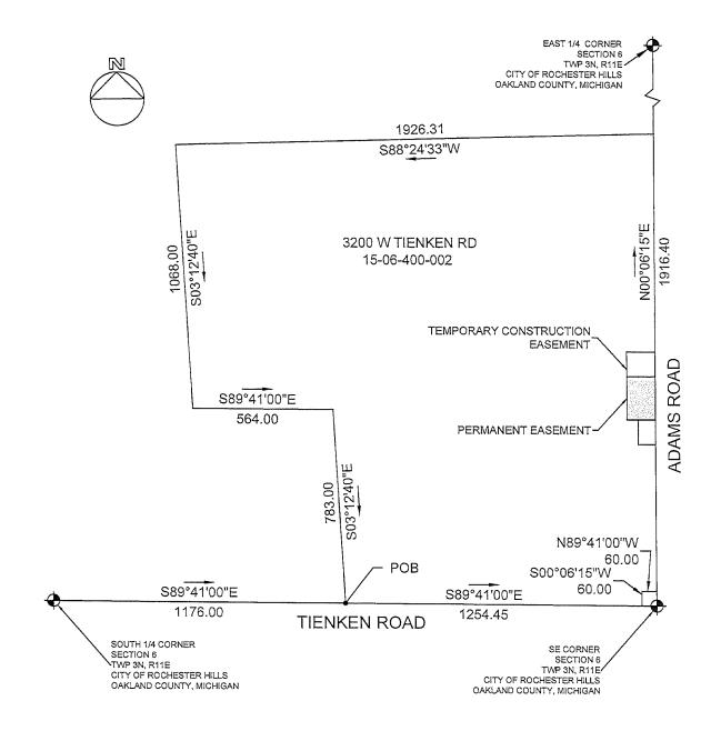
PART OF SE 1/4, SEC 6, T3N, R11E, BEG AT PT DIST S 89°41'00" E, 1176.00 FT FROM S 1/4 COR, TH S 89°41'00" E 1254.45 FT TO SE SEC COR, TH N 00°06'15" E 1916.40 FT, TH S 88°24'33" W 1926.31 FT, TH S 03°12'40" E 1068.00 FT, TH S 89°41'00" E 564.00 FT, TH S 03°12'40" E 783.00 FT TO THE POINT OF BEGINNING, EXC S 60.00 FT OF E 60.00 FT THEREOF, CONTAINING, 70.75 ACRES
