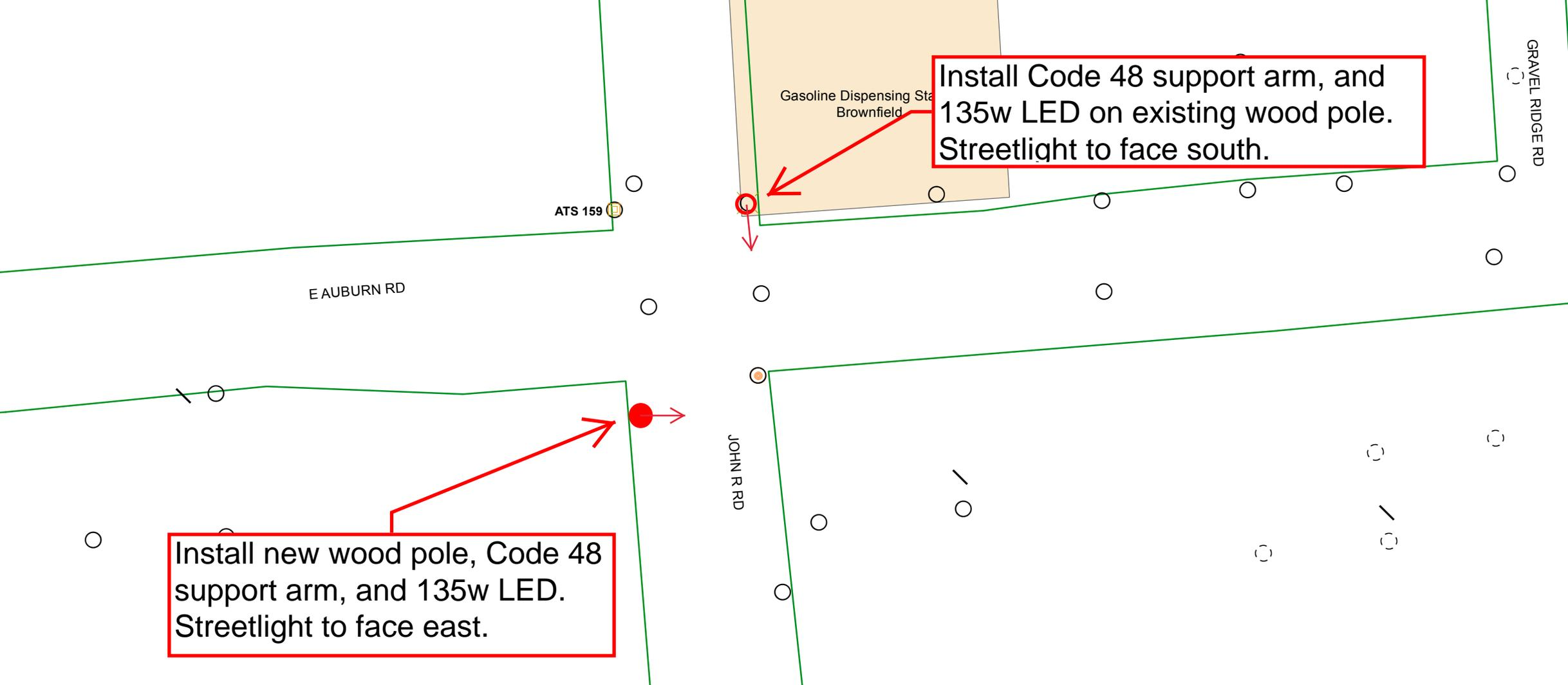
Install Code 48 support arm, and 135w LED on existing wood pole. Streetlight to face south.
