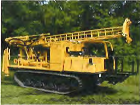
Figure 2.0 ATV-Mounted Drill Rig
