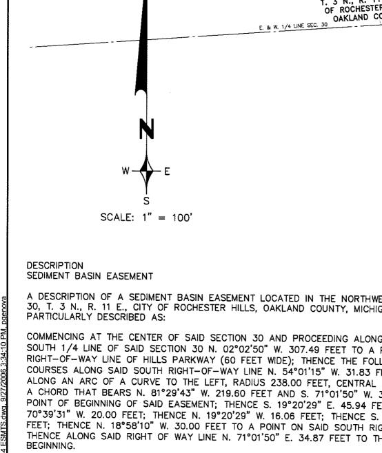
HILLS PARKWAY (60' WIDE) SOUTH R.O.W. LINE R.=238.00' ARC=228.25' △=54°56'55' CHD.=219.60' CHD.BRG.= N81°29'43"W S 71°01'50" W 306.18' N 71°01'50" E N 54°01'15" W 31.83' POINT OF BEGINNING SEDIMENT BASIN EASEMENT 307.49 15.06<sup>-</sup> 16.06<sup>-</sup>-₹ 19"20"29" 8 ≥ ≥ 1/4 LINE SEC. 3 02°02'50" W 70°39'31" 71°01'50" 19°20'29" \ S CENTER OF SEC. 30 1. 3 N., R. 11 E. CITY OF ROCHESTER HILLS, E. & W. 1/4 UNE SEC. 30 OAKLAND CO., MI. SEC. 1/4 LINE
