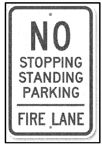
FIRE LANE SIGN DETAIL N.T.S. Provide at spaces per fire department requirements
