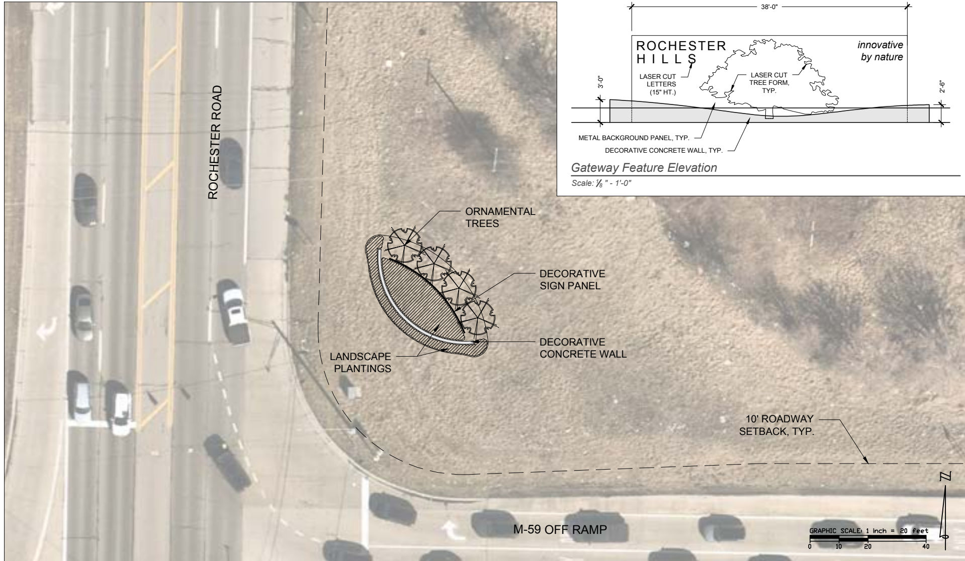
Rochester Road & M-59 - "Super" Primary Gateway Scale: 1" = 20'-0"
