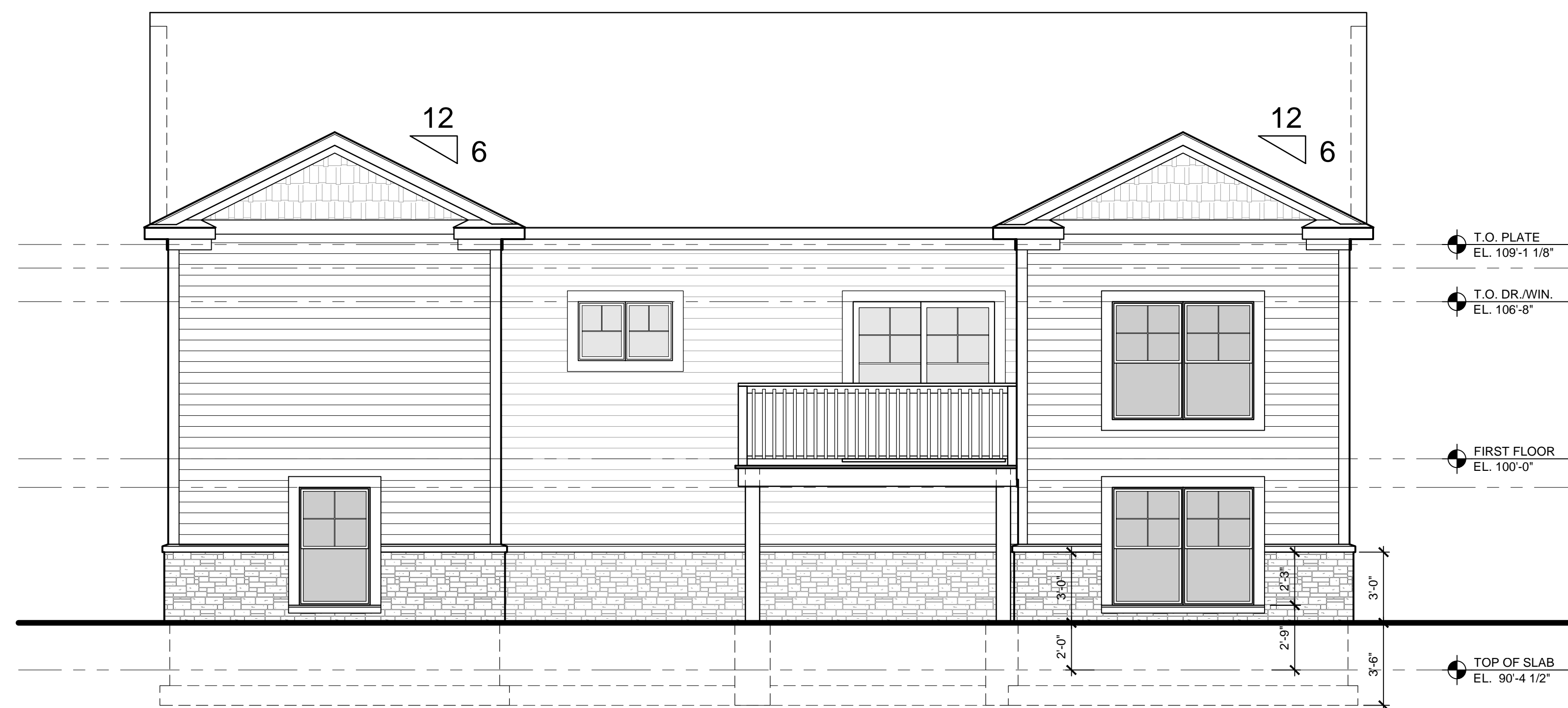
3 REAR ELEVATION - Chelsea Deep SCALE: 1/4" = 1'-0" DAYLIGHT ELEVATION
