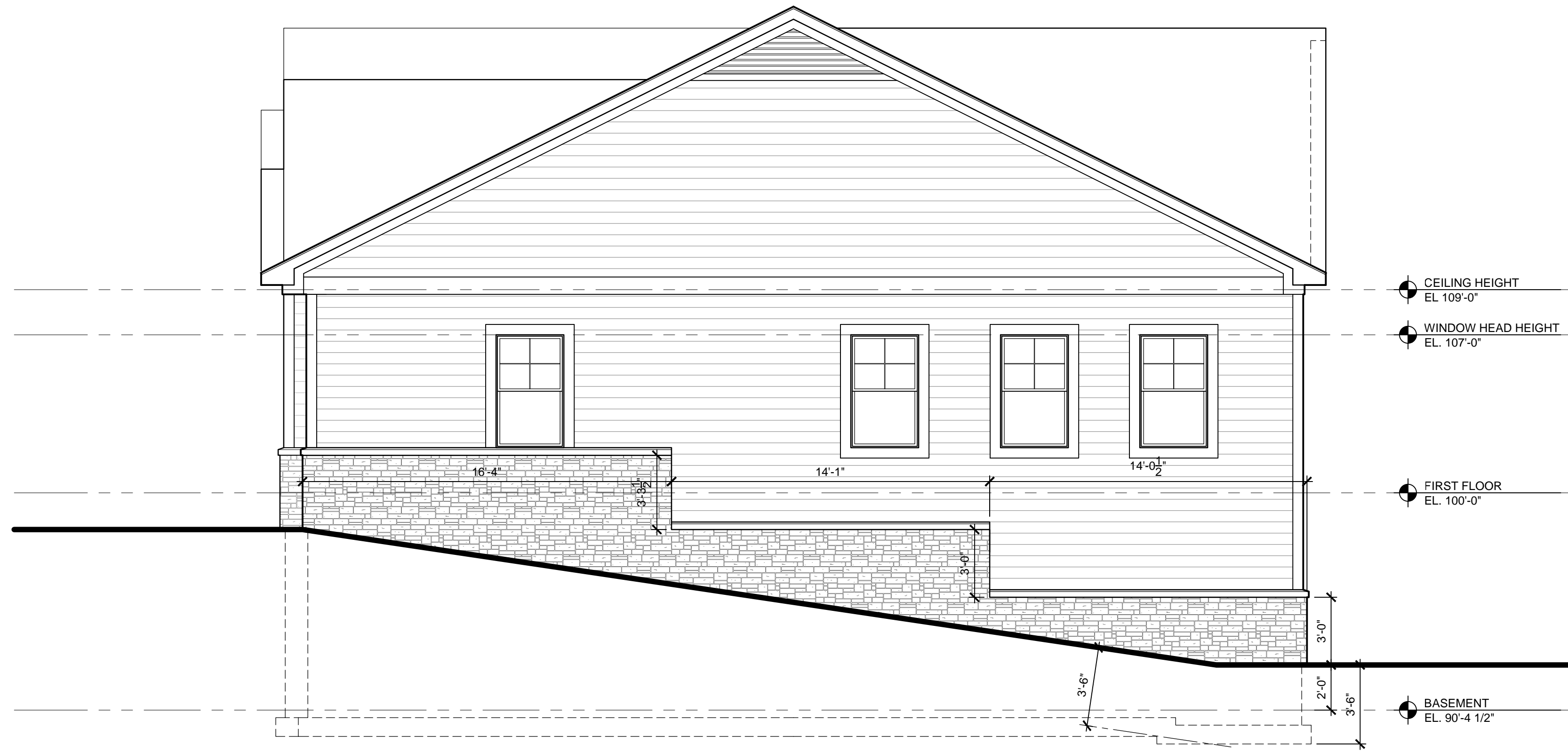
HURON SIDE ELEVATION DAYLIGHT ELEVATION SCALE: 1/4" = 1'-0"
