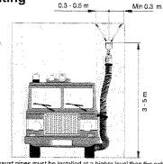
N.B. The nozzle for high level (HL) exhaust pipes must be installed at a higher level than the exhaust pipe. The nozzle must be pulled downwards at connection, which will activate the balancer.
