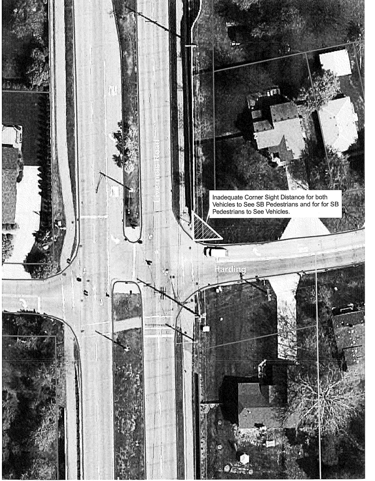
Inadequate Corner Sight Distance for both Vehicles to See SB Pedestrians and for for SB Pedestrians to See Vehicles.
