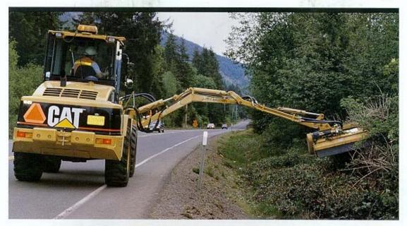
The IT14G is the ideal platform for the Little Industries Brushcutter. Greater visibility to the mower, better sight line, versatility, weight of the machine and hystat transmission result in increased operator confidence and productivity.
