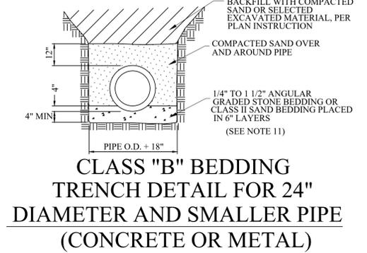
CLASS "B" BEDDING TRENCH DETAIL FOR 24" DIAMETER AND SMALLER PIPE (CONCRETE OR METAL)
