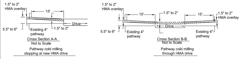
Cold milled section of existing pathway to be replaced with 1.5" to 2" HMA overlay
