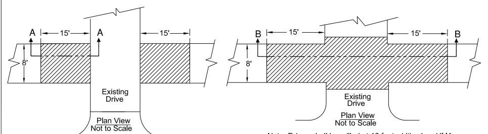
Note: Drives shall be milled at 10 foot width when HMA pathway is resurfaced through the drive (as directed by engineer).
