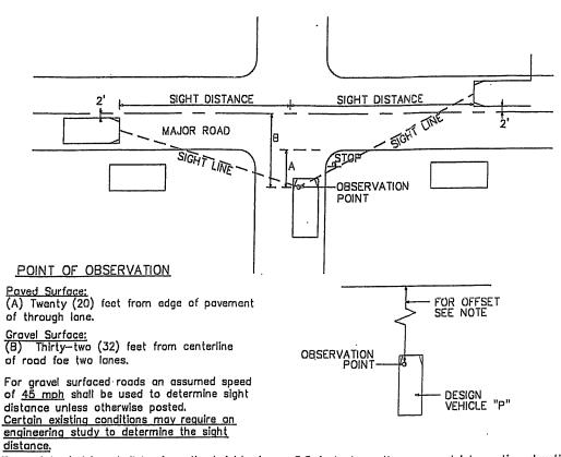
The point of vision shall be from the height of eye, 3.5 feet above the proposed intersecting elevation to a height of object 3.5 feet above the existing or proposed road centerline and shall be continuously visible within the specified limits.
