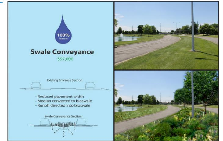
Above right shows the current conditions of the Clinton Township Municipal Complex entrance with existing turf grass with nearly zero water treatment and conveyance. The bottom right concept graphic depicts raingarden installation into the swaled area with 100% stormwater conveyance and treatment of nutrient run off.
