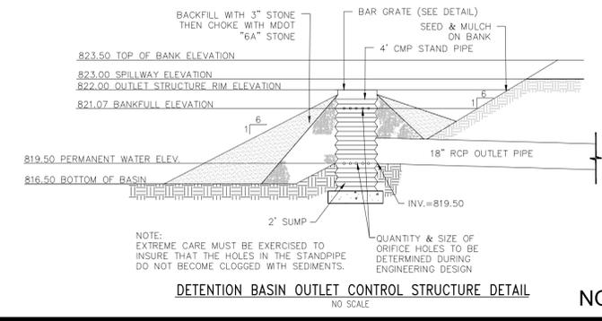
NOTE: EXTREME CARE MUST BE EXERCISED TO INSURE THAT THE HOLES IN THE STANDPIPE DO NOT BECOME CLOGGED WITH SEDIMENTS.
