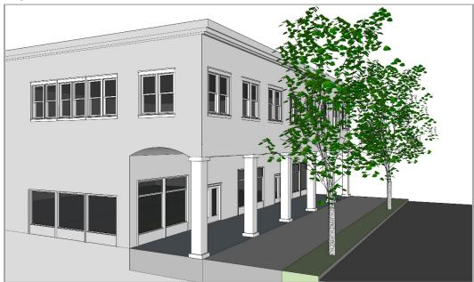
Below: Arcade section view shows the recessed pedestrian walkway and the upper floor area above. The entire structure is on private property, and the columns and upper floors extend to the front lot (build to) line.
