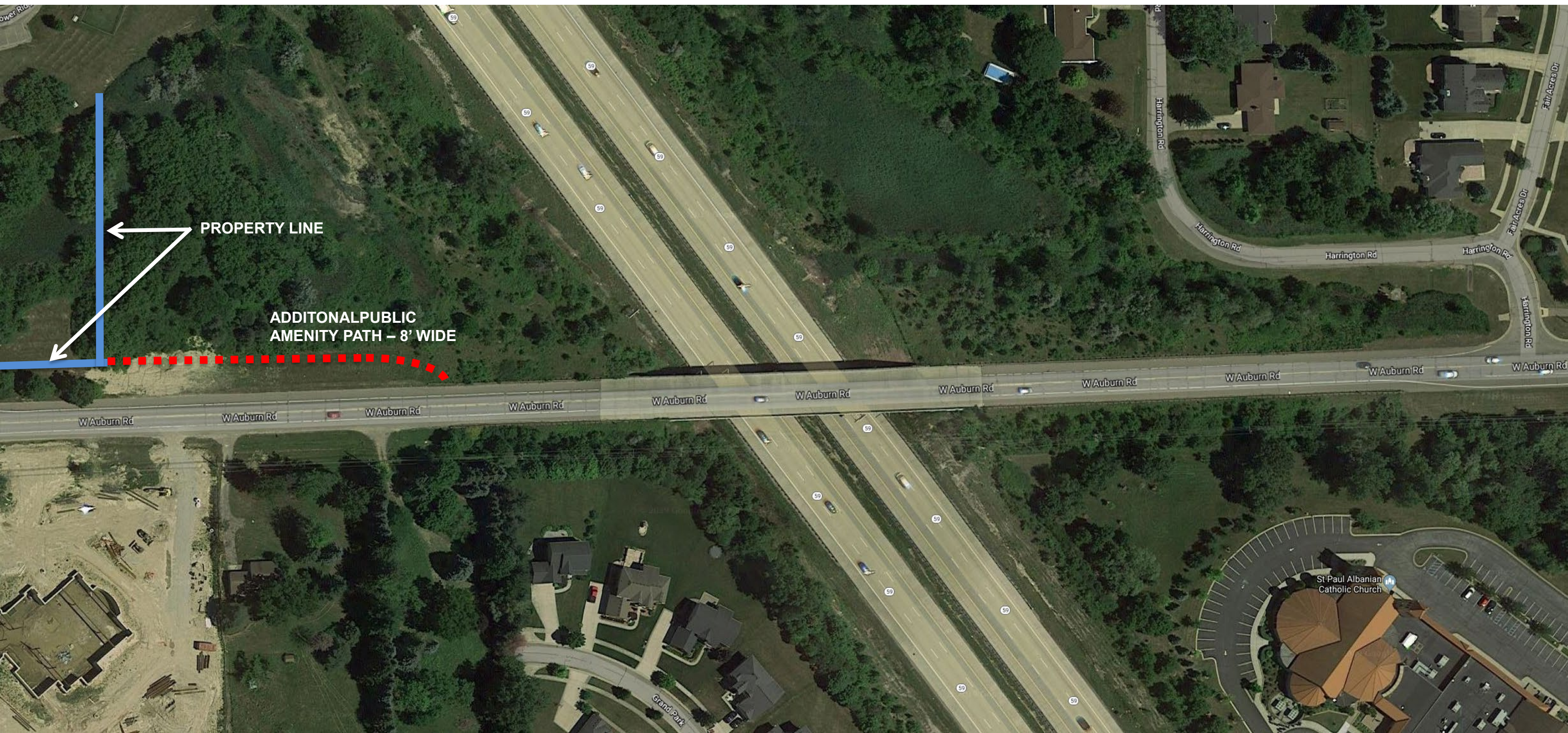
ADDITIONAL 8' WIDE SAFETY PATH – 381 FEET LONG
