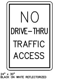
7'-0" MOUNTING HEIGHT NO DRIVE THRU ACCESS SIGN DETAIL NOT TO SCALE
