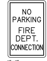
12" x 18" RED ON WHITE REFLECTORIZED 7'-0" MOUNTING HEIGHT NO PARKING-FDC SIGN DETAIL
