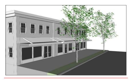
Below: Section view of shopfront illustrating relationship of storefront to pedestrian walkway. Street trees and awnings provide protection from the elements and reduce the impact of high temperatures during warm weather months.
