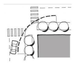
Figure 4. Effective Turning Radius
