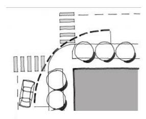
**Figure 4. Effective Turning Radius**
