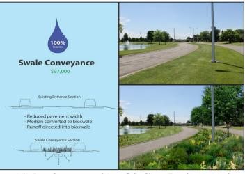
Above right shows the current conditions of the Clinton Township Municipal Complex entrance with existing turf grass with nearly zero water treatment and conveyance. The bottom right concept graphic depicts raingarden installation into the swaled area with 100% stormwater conveyance and treatment of nutrient run off.
