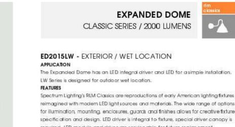
Spectrum Lighting's RLM Classics are reproductions of early American lighting fixtures reimagined with modern LED light sources and materials. The wide range of options for illumination, mounting, enclosures, guards and finishes allows for creative fixture specification and design. LED driver is integral to fixture, special driver canopy is required. LED module and driver are serviceable for future replacement.
