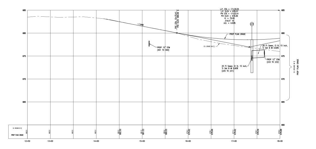
[23] STA 17+39.05, 0.0' L 48" DIA CATCH BASIN, COVER B T/CAST 678.57 15" INV NE 673.97 15" INV SW 673.87 15" INV NW 674.76 ARCHITECTS ENGINEERS PLANNERS
