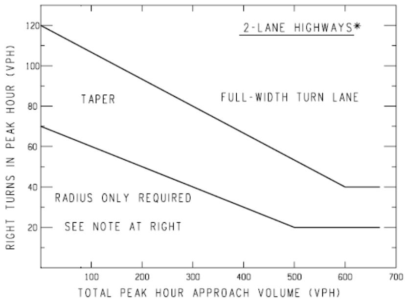
NOTE: For posted speeds at or under 45 mph, peak hour right turns greater than 40 vph, and total peak hour approach less than 300 vph, adjust right turn volumes.
