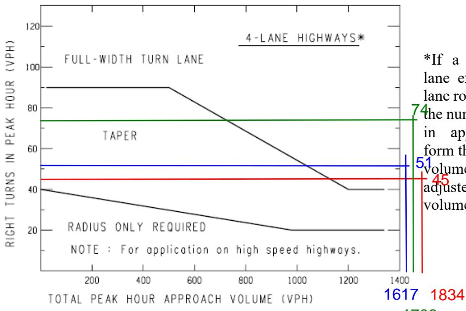
\*If a center left-turn lane exists (ie 3 or 5 lane roadway), subtract the number of left turns in approach volume from the total approach volume to get an adjusted total approach volume.
