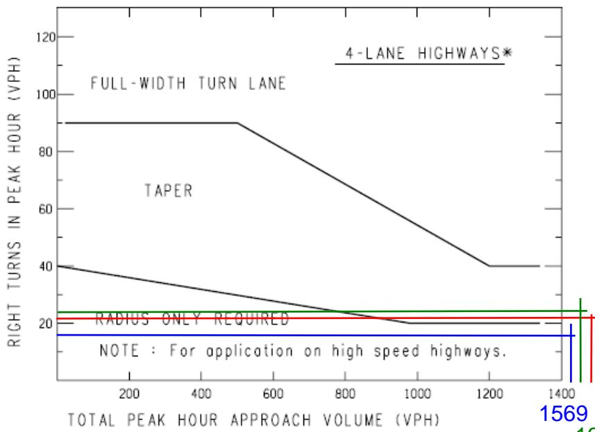
\*If a center left-turn lane exists (ie 3 or 5 lane roadway), subtract the number of left turns in approach volume from the total approach volume to get an adjusted total approach volume.
