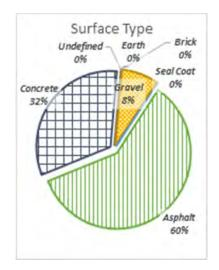
Figure 2: Pavement type by percentage maintained by CoRH. Undefined pavements have not been inventoried in CoRH's asset management system to date, but will be included as data becomes available.
