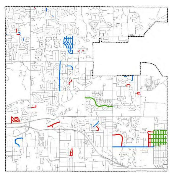
Figure 5 : Map illustrating planned projects for pavement assets. 2022 planned projects are in blue, 2023 in red, and 2024 in green.
