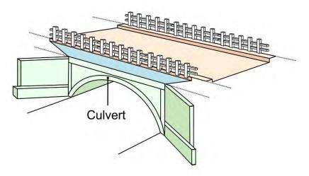
Figure C-1: Diagram of a culvert structure
