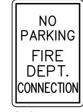
12" x 18" RED ON WHITE REFLECTORIZED 7'-0" MOUNTING HEIGHT NO PARKING-FDC SIGN DETAIL
