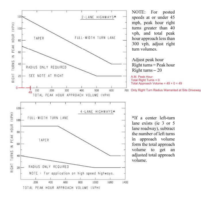
Sample Problem: The Design Speed is 55 mph. The Peak Hour Approach Volume is 300 vph. The Number of Right Turns in the Peak Hous is 100 vph. Determine if a right turn lane is recommended.
