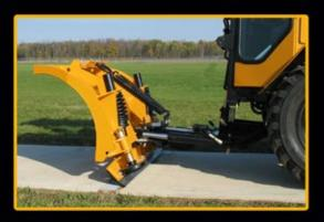
Winter can take a toll on sidewalks creating uneven surfaces which makes plowing snow difficult. The Double Trip Sidewalk Plow was built for municipalities that have a significant number of toe trips resulting in constant plow tripping. The double trip system trips the mouldboard 35° and the cutting edge 40° which protects both the plow and the MT from damage when obstacles are encountered.
