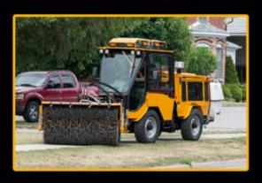
The Power Angle Sweeper can be used to perform a wide variety of tasks every month of the year making it one of the most cost-effective and versatile attachments to own. In addition to sweeping sand, gravel or other debris from sidewalks, parking lots, cul de sacs, intersections or other confined areas, the sweeper can also be used to dethatch large lawns and playing fields in the summer or remove snow from sidewalks in the winter.
